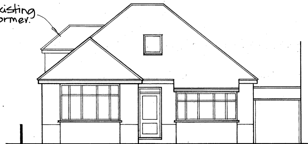
EXISTING FRONT ELEVATION
