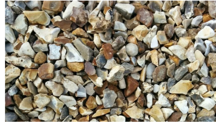
Rear Garden Log Store Enclosure & Access Path: 6-10mm flint/Cotswold gravel, 25-40mm depth; permeable geotextile underlay; untreated steel edging. Supplier: Contractor to propose local supplier
