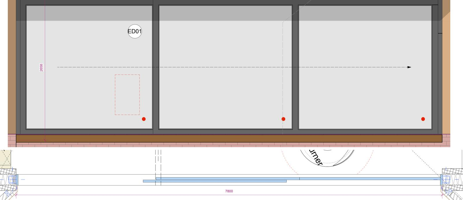
New Windows & Doors (max U value = 1.2 W/m<sup>2</sup>k) Paint finish: Powder color coated grey. RAL TBC
