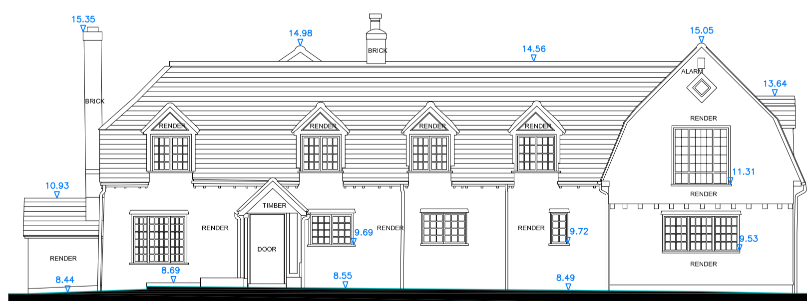
Front Elevation Scale 1:100
