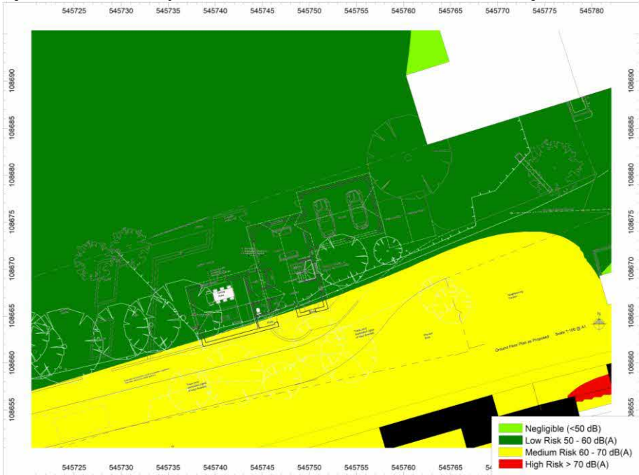
Figure 6-2: ProPG Initial daytime site noise risk assessment (Contours at 1.5 m above ground level)
