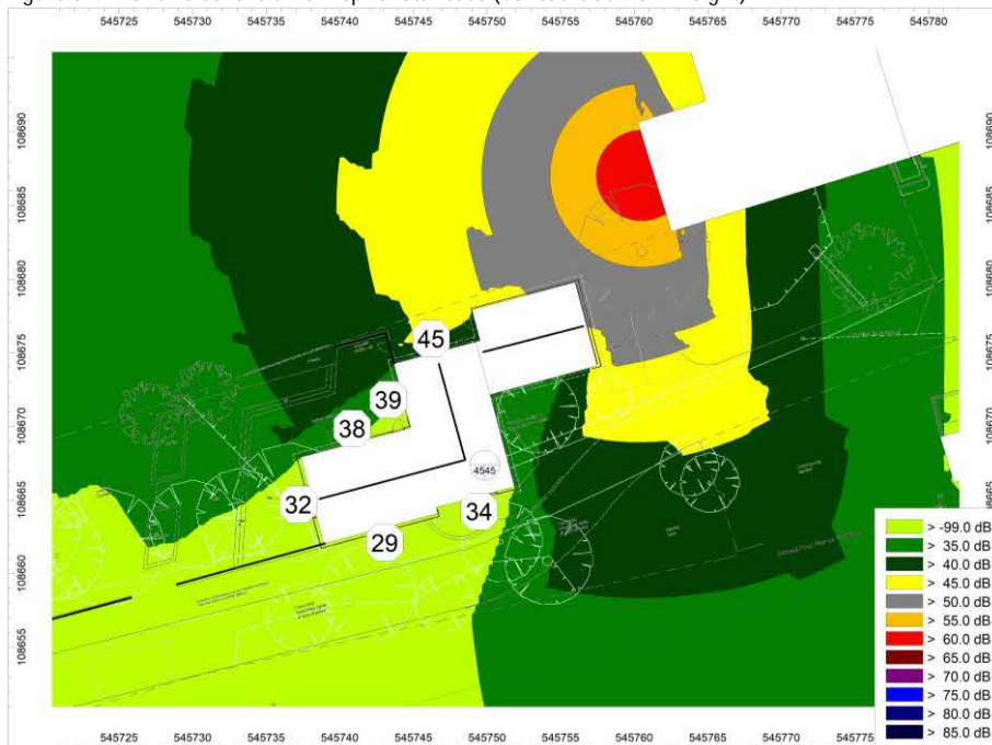
Figure 5-4: Plant noise levels from Spiral Staircase (Contours at 4.0 m height)
