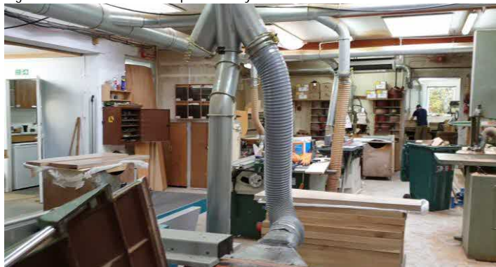
Figure 5-2: Internal workshop extract system
