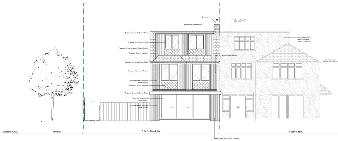
Proposed Building Rear Elevation/ Section EE Scale 1:100
