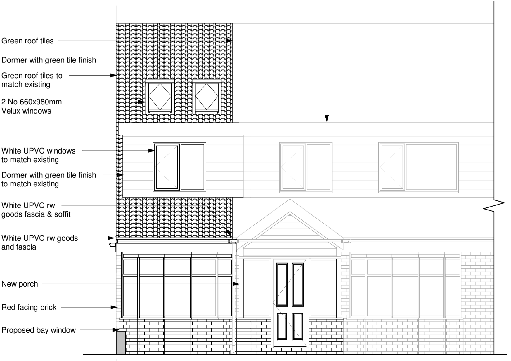
1 Front Elevation - Proposed 1 : 50
