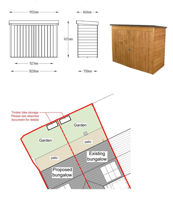
Timber cycle storage to be located as per drawing extract below:
