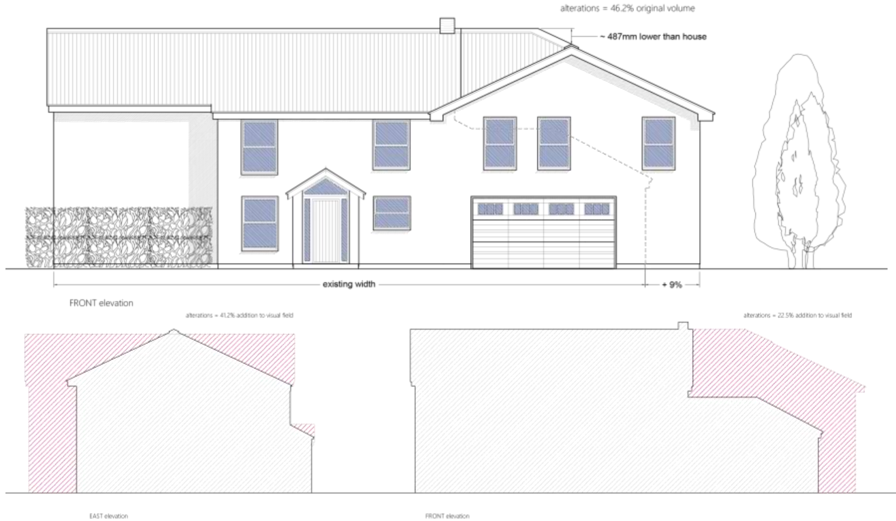
Figure 15 - Developed option 2 (+46% existing volume & 22.5% area of front elevation)
