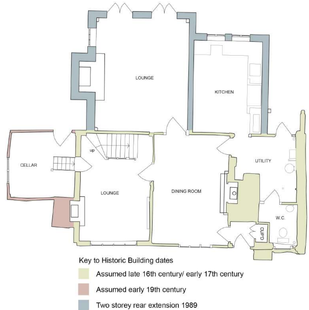
17. Diagram to show dating of the historic and more modern fabric at Bridge Cottage
