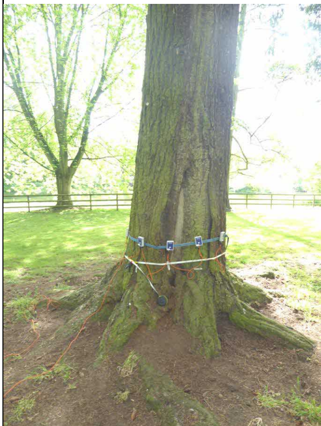
Base of T361 left. Tomograph of base showing generally sound wood (dark) in centre. Green area is the pocket where lightning entered rootzone.
