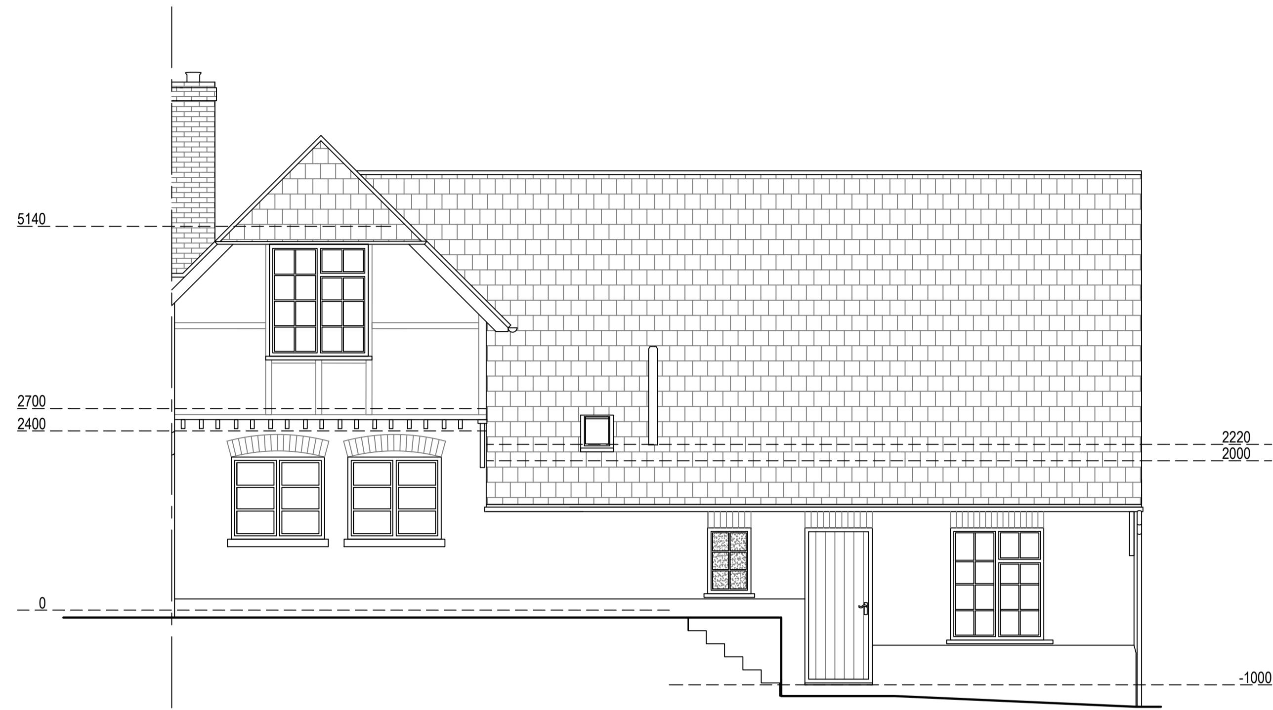
Existing Northwest Elevation Scale 1:50
