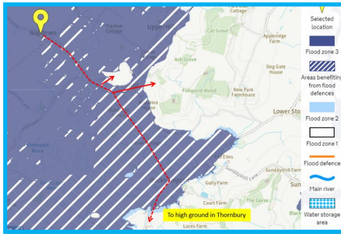
Fig 17 Proposed flood evacuation route, moving away from the source of flooding within defended areas, including routes to local hills.
