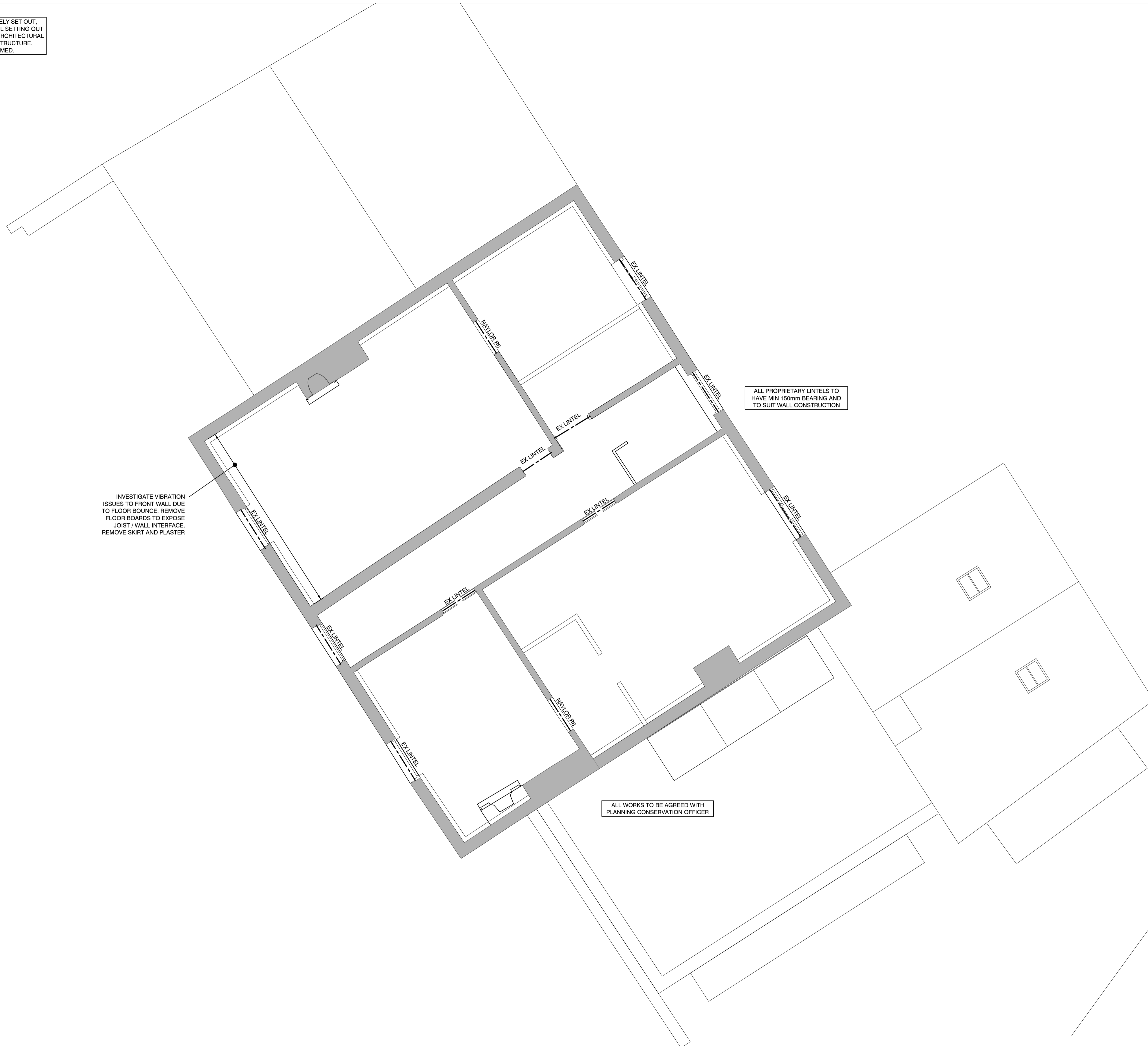
PROPOSED SECOND FLOOR LAYOUT INDICATING STRUCTURE OVER 1:50
