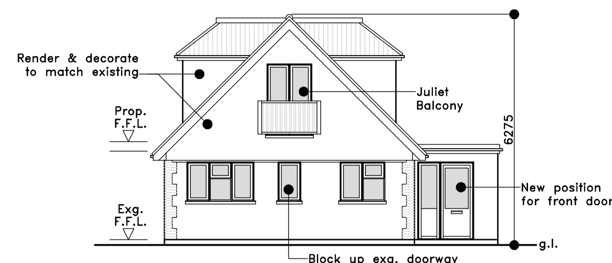
PROPOSED FRONT ELEVATION NORTH
