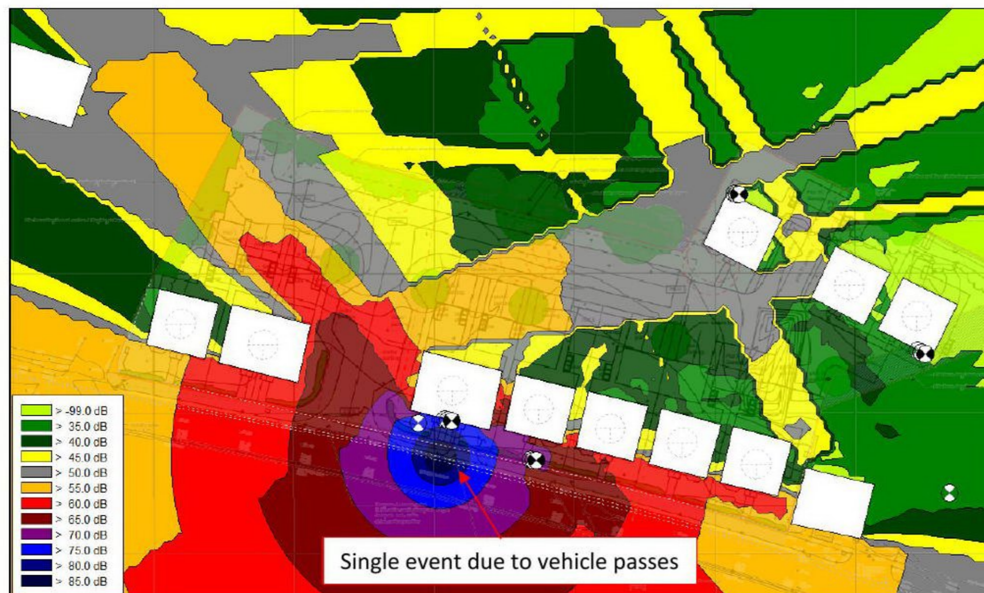
Figure 6: Plan viewing L_{AFmax} sound contours at 4 m above ground due to vehicle passes, affecting proposed houses directly facing Barrington Road
