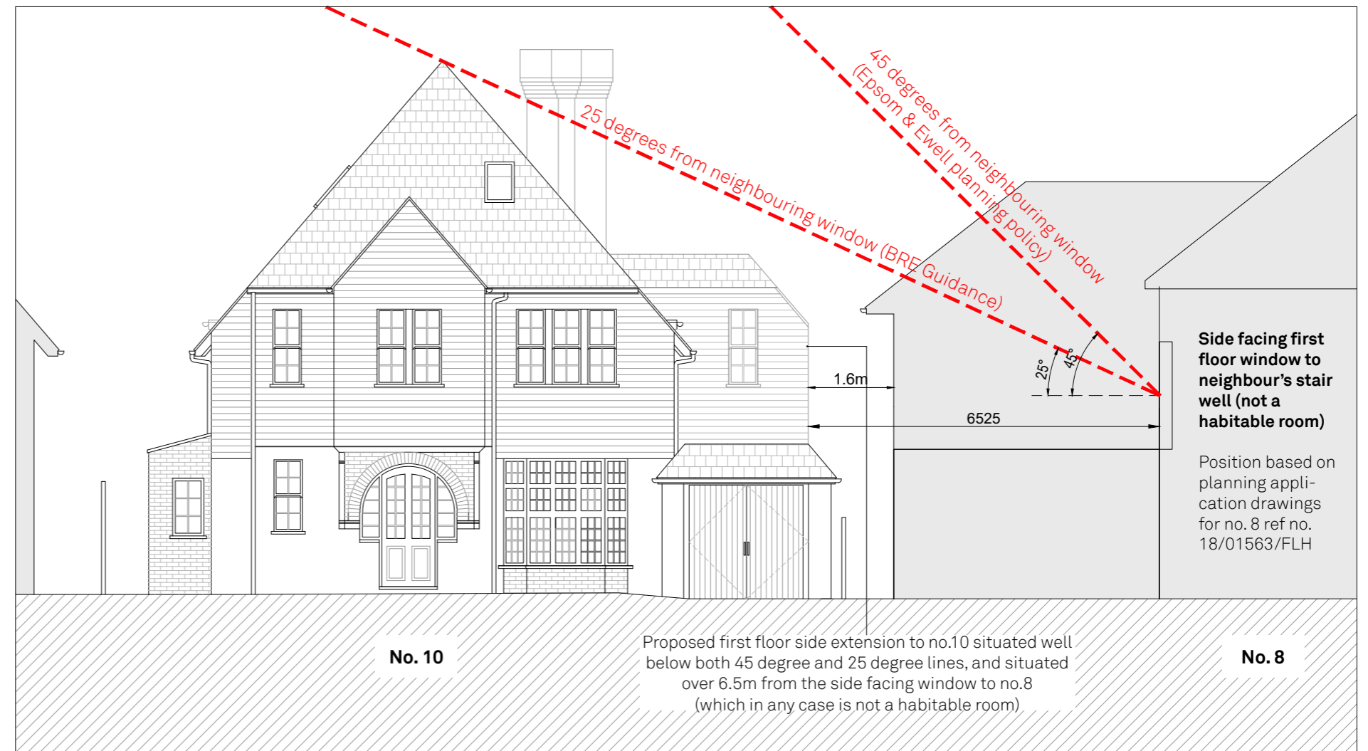
Front elevation diagram demonstrating that the proposed first floor side infill extension to No. 10 Kingsdown Road shall have no discernible impact upon the side facing first floor stairwell window to the neighbouring property at No.8 Kingsdown Road Scale 1:100 at A3
