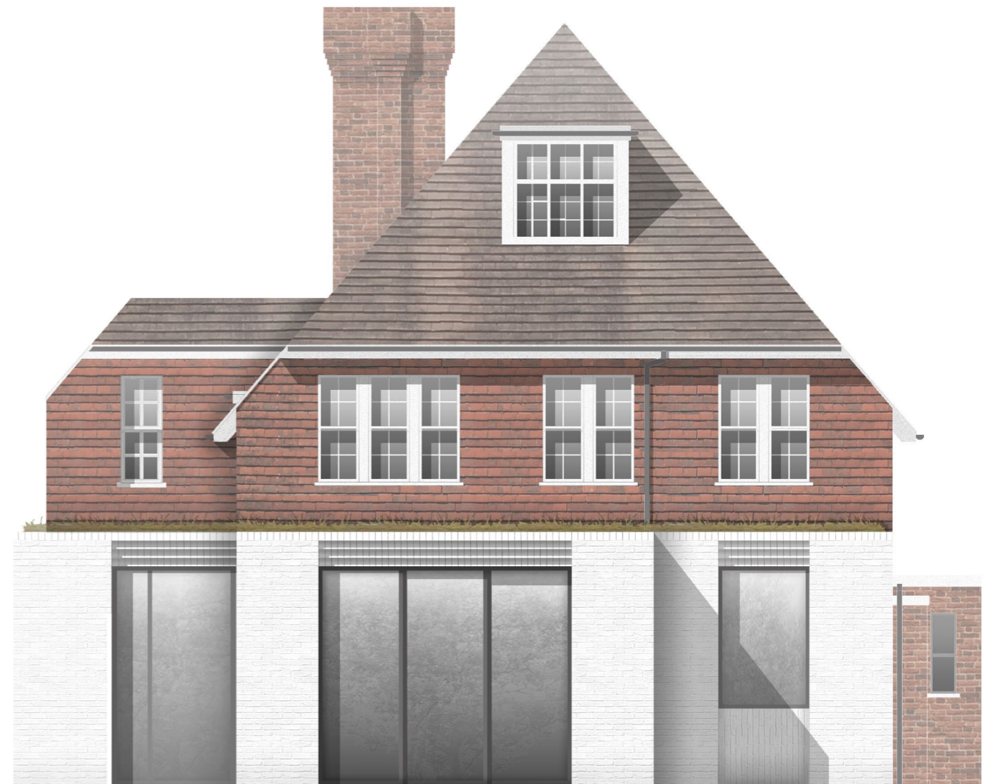
Rear elevation: Proposed extensions, complimentary to the character of the existing house
