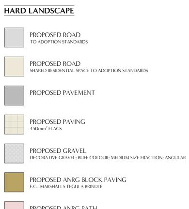
PROPOSED ANRG PATH SELF BINDING AGGREGATE WITH TIMBER EDGE
