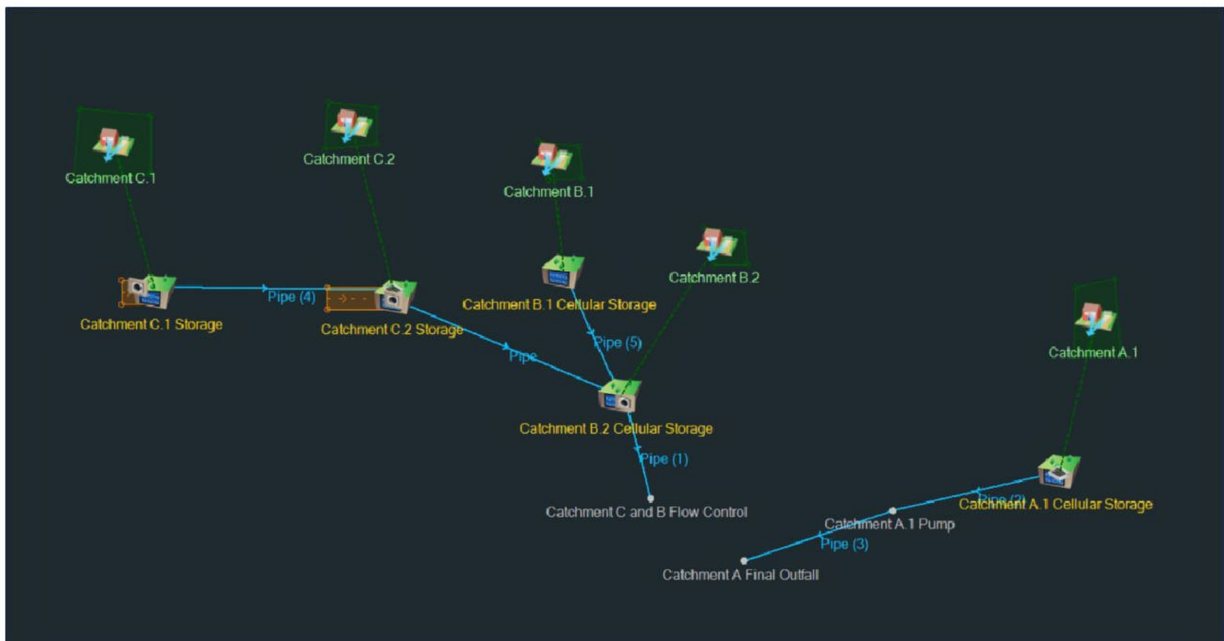
Figure 7 Schematic of InfoDrainage network
