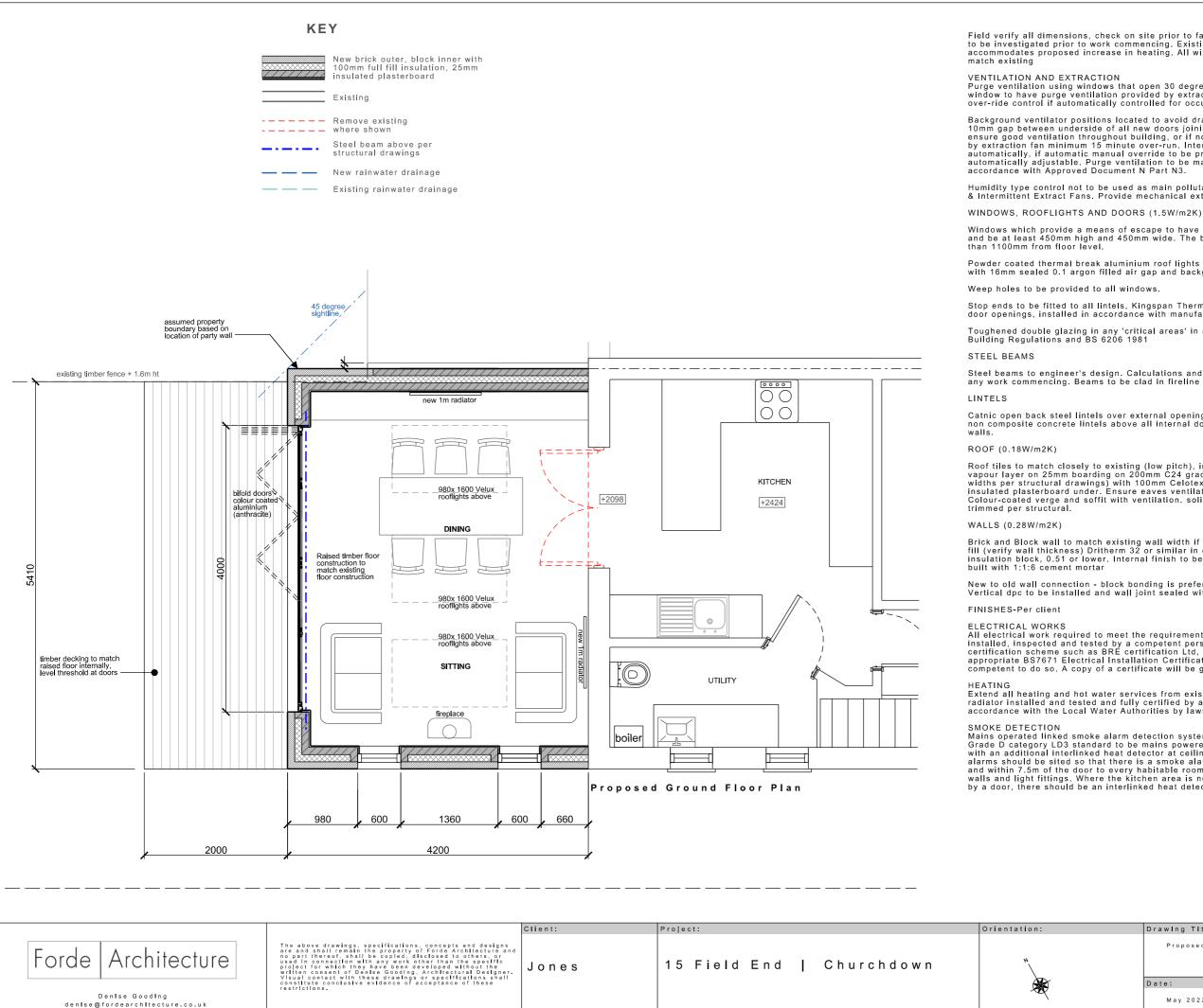
Field verify all dimensions, check on site prior to fabrication and erection. All existing services on site to be investigated prior to work commencing. Existing heating system to remain, verify capacity accommodates proposed increase in heating. All wiring and pipes to be hidden. Skirting boards to
