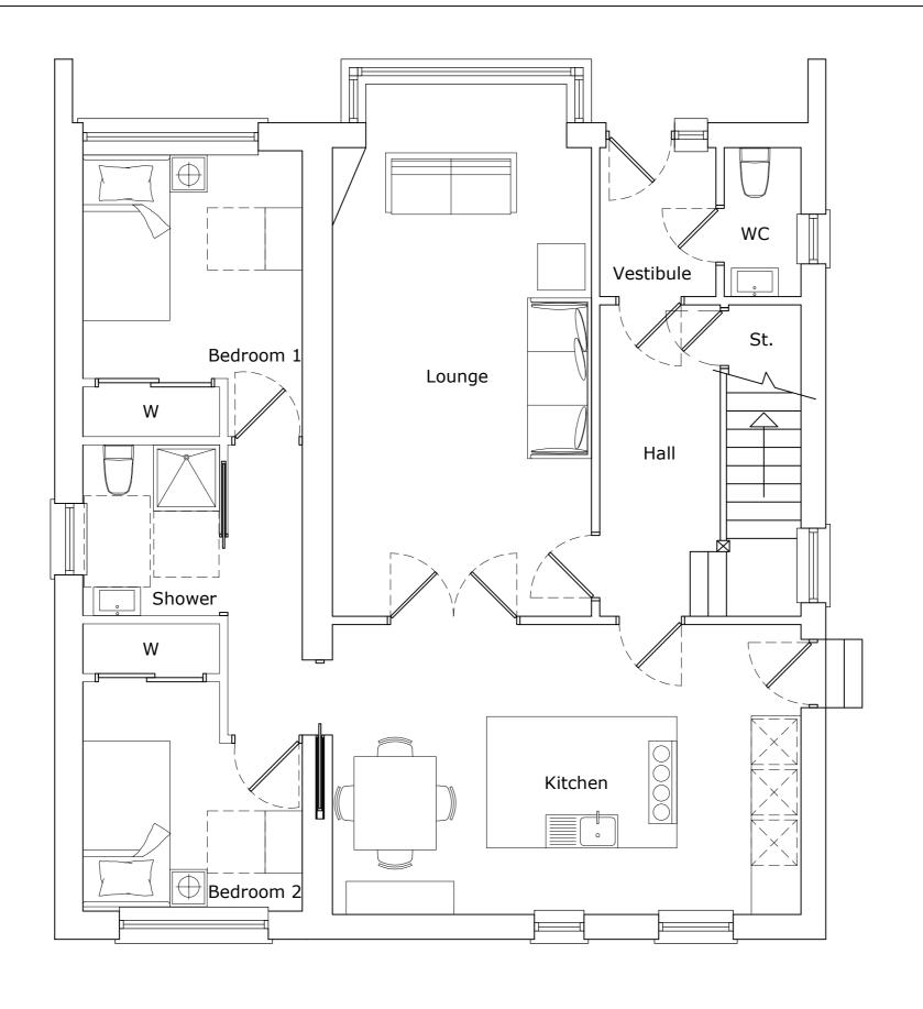
Proposed Ground Floor Plan Scale 1:50
