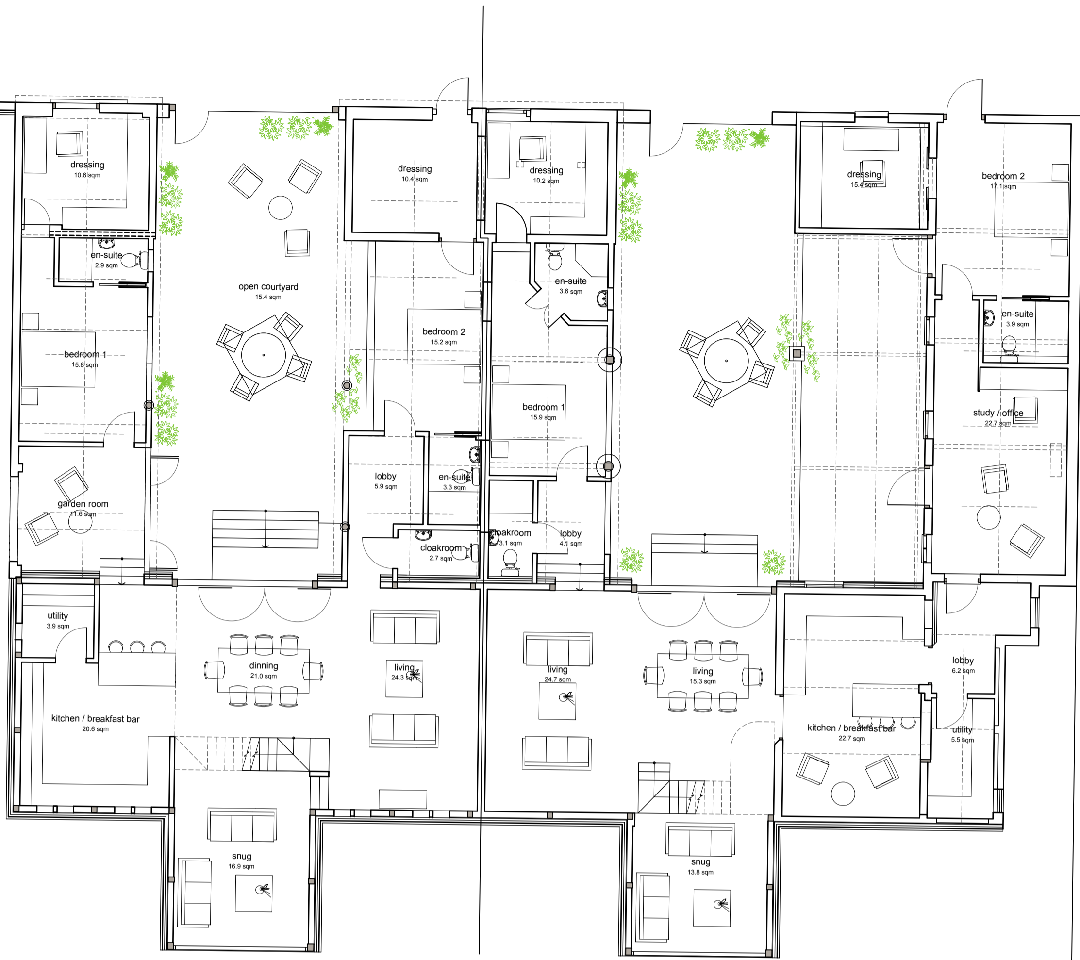
plot 3 proposed ground floor plan 1:100 Total Ground Floor Gross Internal Area = 170.5 m 2 [1835 sqft] Total Gross Internal Area = 213.1 m 2 [2293 sqft]
