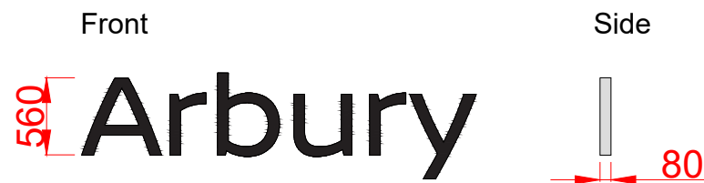
Sign D: Dealer Name Size 5 Individual 3D letters Face Illumination: Internally Illuminated with white LEDs Material: 1mm Hairline S/S Returns 4mm Black/White Acrylic Front Face Scale 1:50 @ A3
