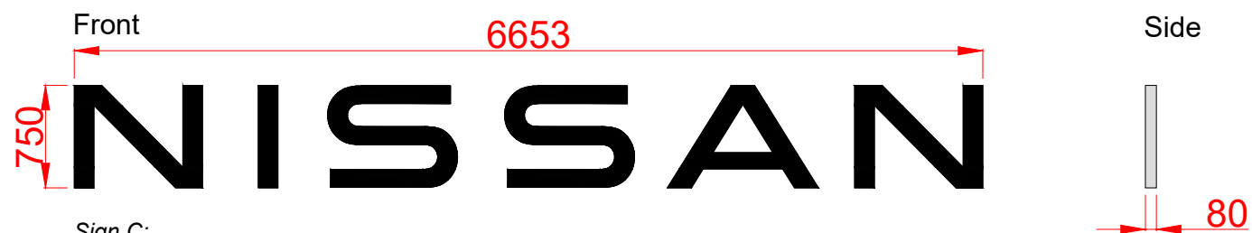
Sign C: Nissan Wordmark Size 5 Individual 3D letters Face Illumination: Internally Illuminated with white LEDs Material: 1mm Hairline S/S Returns 4mm Black/White Acrylic Front Face Scale 1:50 @ A3
