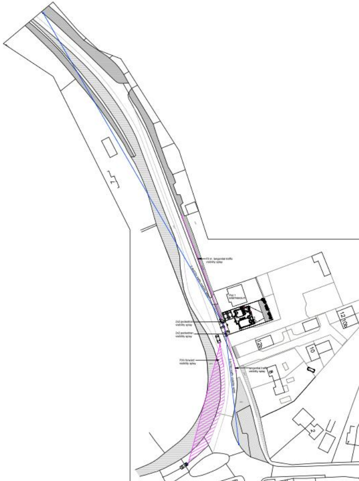
Fig 13. Proposed Site Plan, showing traffic visibility splays
