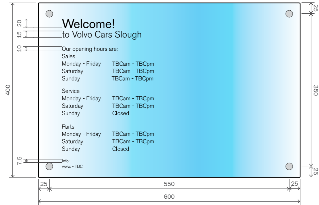
FRONT ELEVATION scale 1:5
