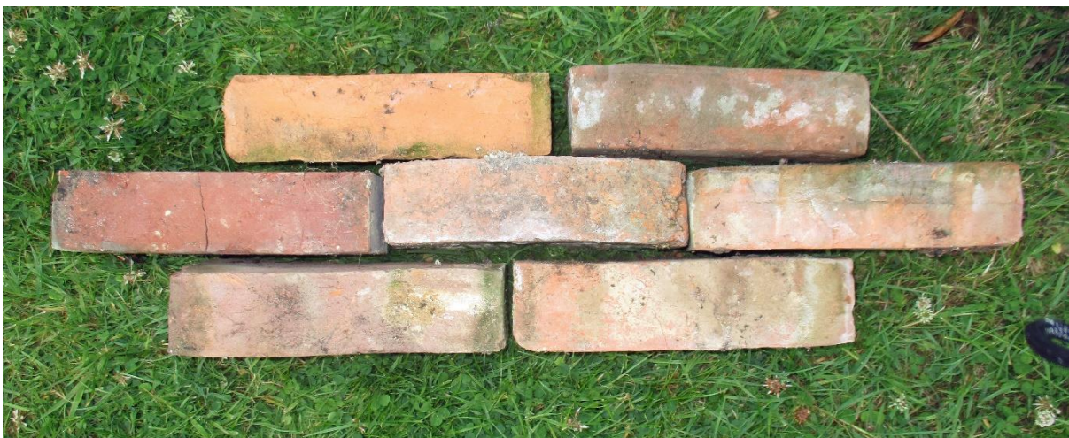
Salvaged handmade clay bricks
