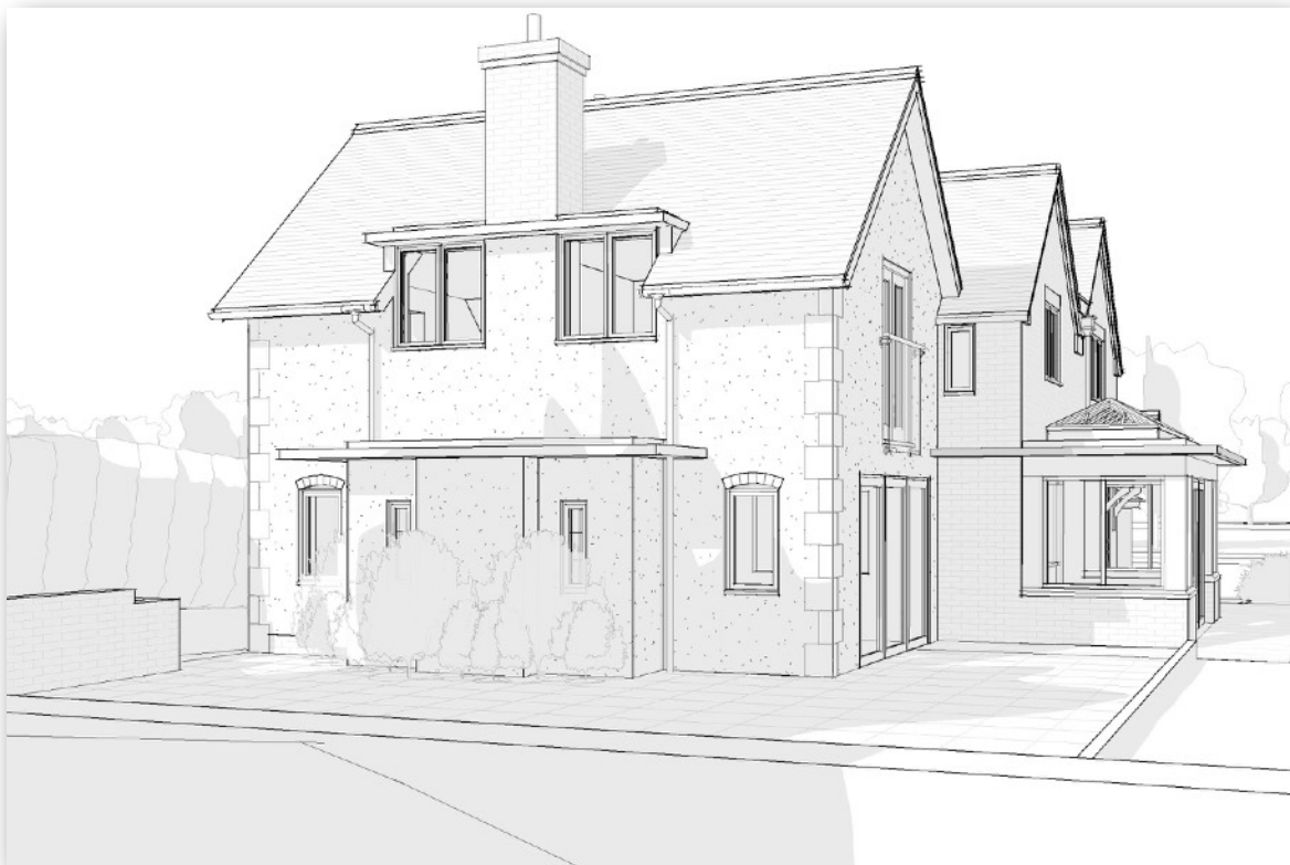
The above computer-generated image shows the proposed design viewed from the east, with the white UPVC conservatory fully removed, and the modern out of keeping brickwork covered with a more appropriate locally acceptable off-white render.
