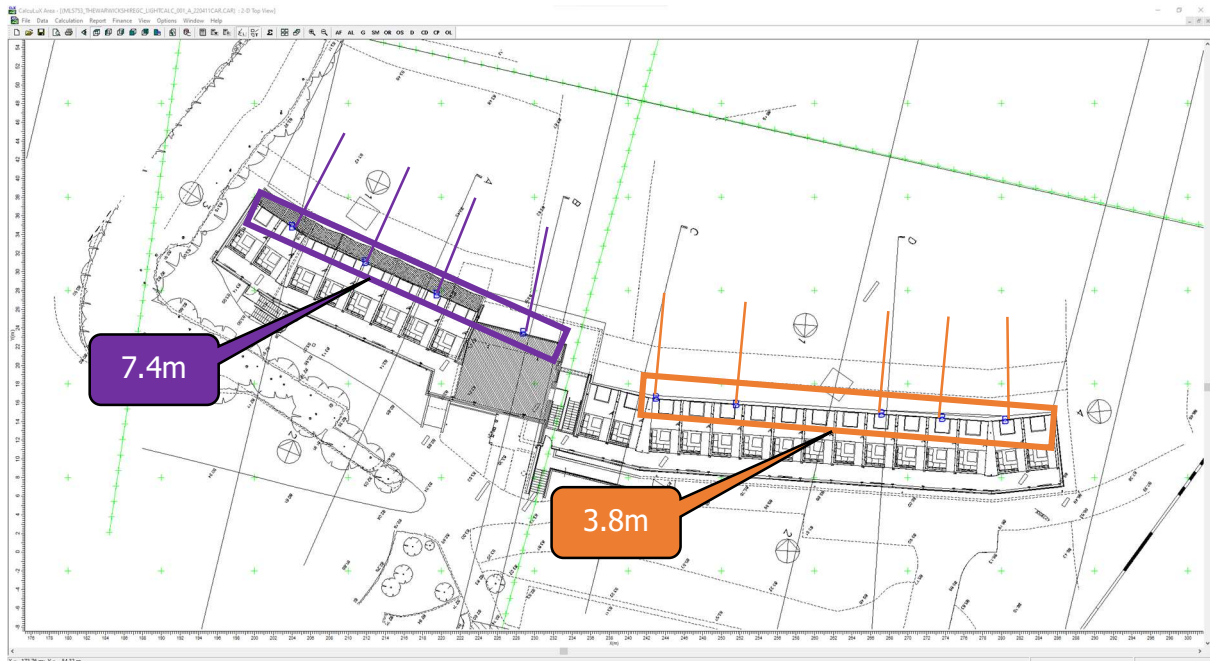
Figure 4 - Proposed layout and mounting height of lights
