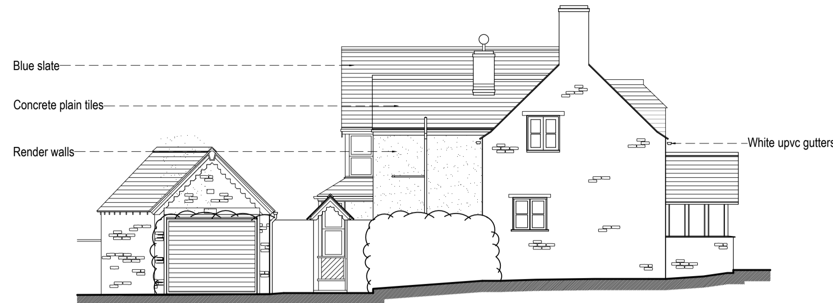
Existing West (Side) Elevation 1:100 @ A1
