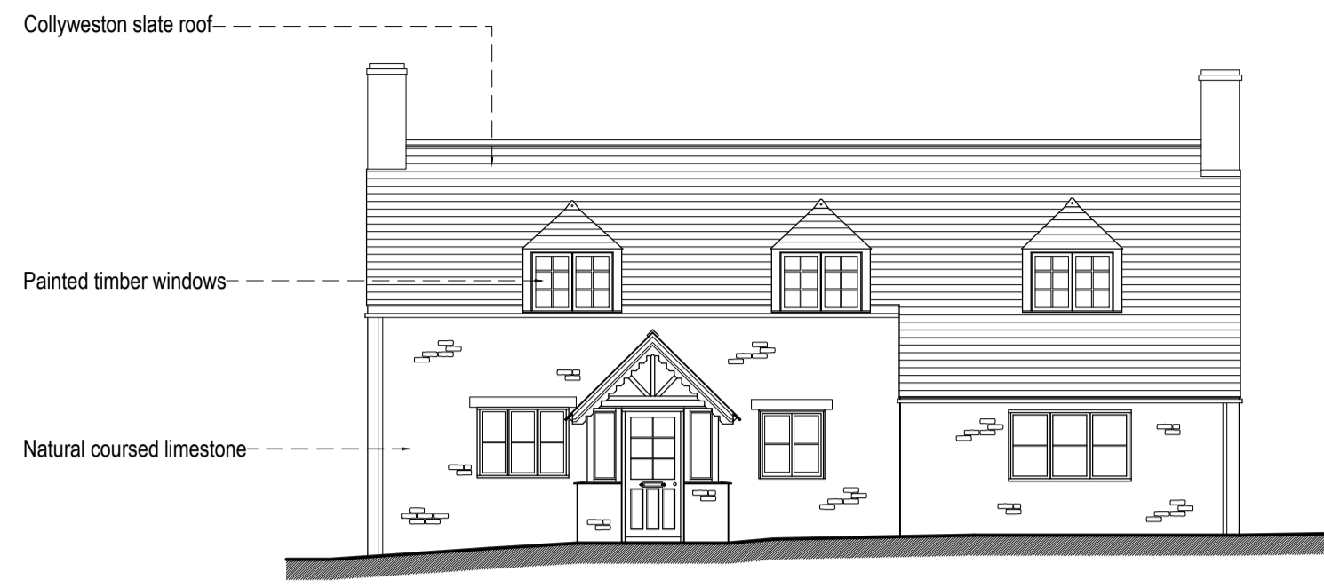
Existing South (Front) Elevation 1:100 @ A1
