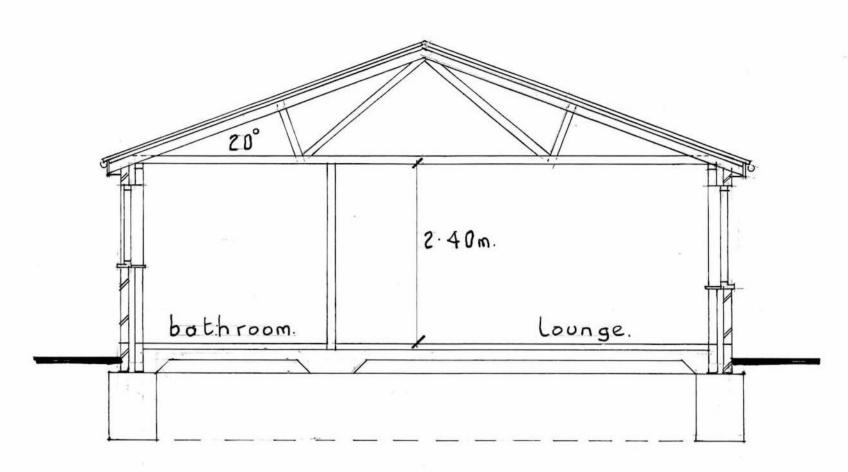
Foundations. - to be 600mm. wide x I metre deep trench fill concrete founds to all new external walls. Final depth of founds agreed on site with Building Inspector. Internal block wall built off thickened out concrete floor slab.
