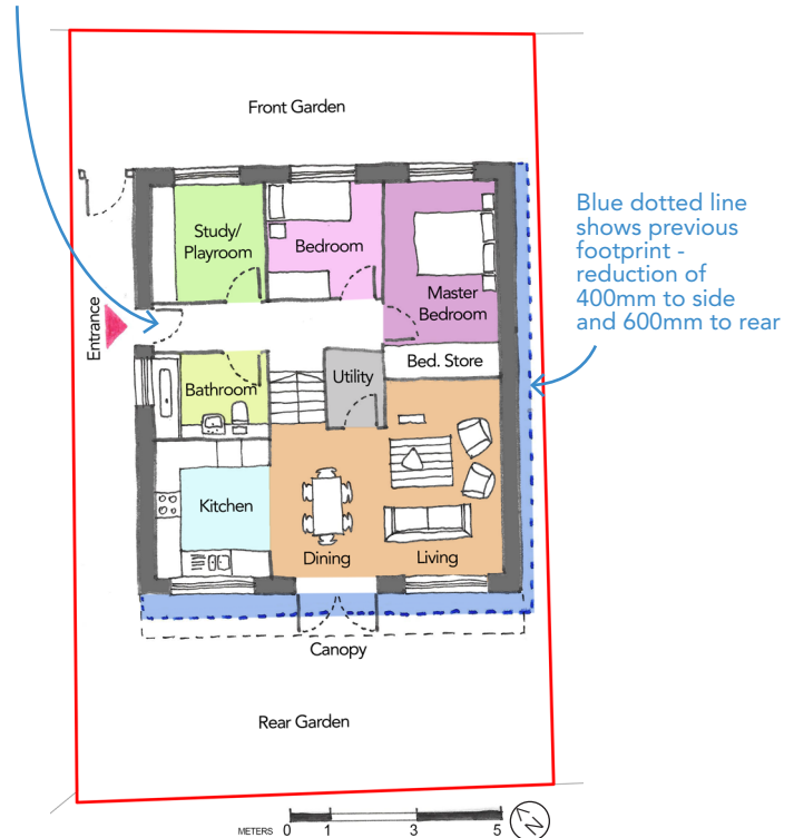
Revised Ground Floor Arrangement Following Pre-Application meeting
