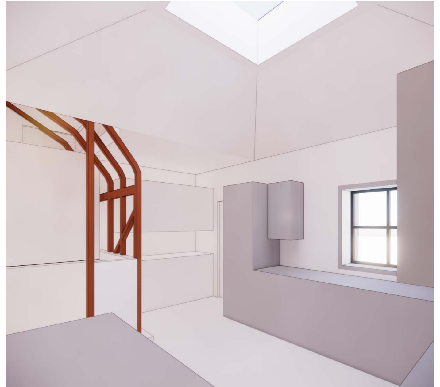
Proposed Kitchen - 3D views showing the existing timber frame, stripped of its plaster and thatch, incorporated to create an entrance to the kitchen.
