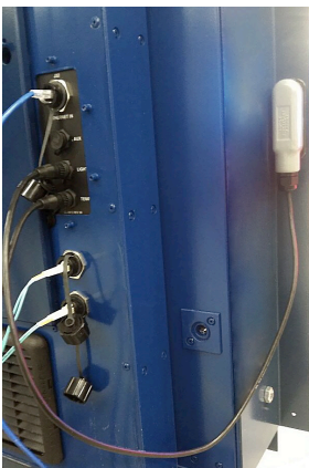
Image 1 – example ambient light sensor
