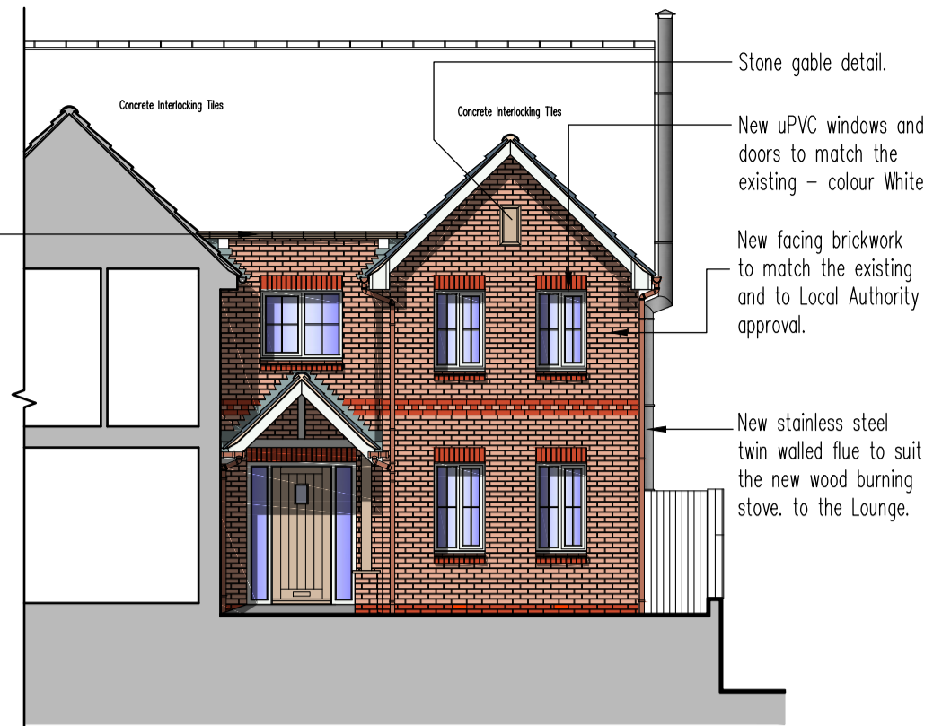
PROPOSED NORTH WEST SECTION/ELEVATION (1:100)
