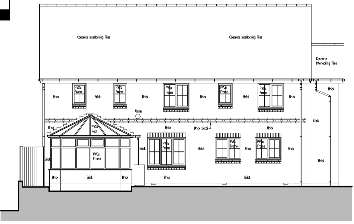
EXISTING SOUTH EAST ELEVATION (1:100)
