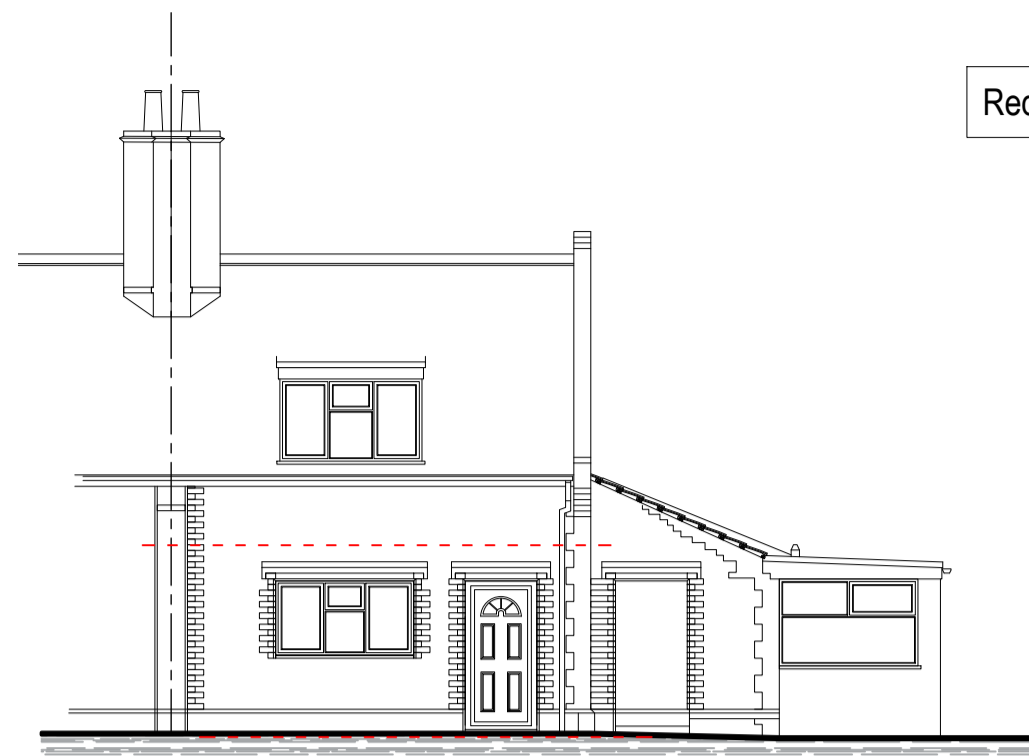
FRONT ELEVATION AS EXISTING 1/100
