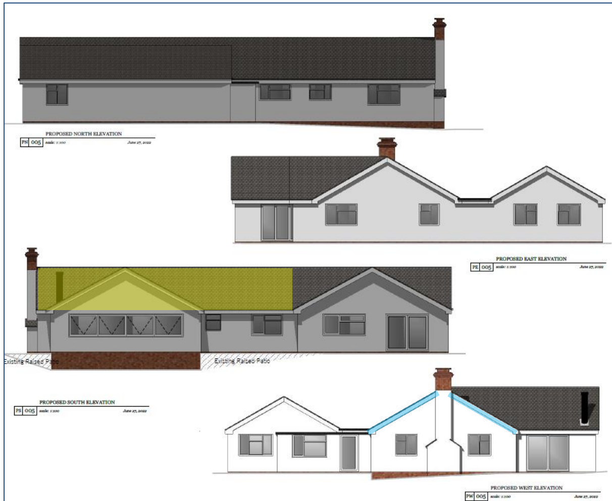
Plan 6. Barge boards and tile verge areas with existing gaps to be retained (blue shading). Roof void space to be retained (yellow shading)
