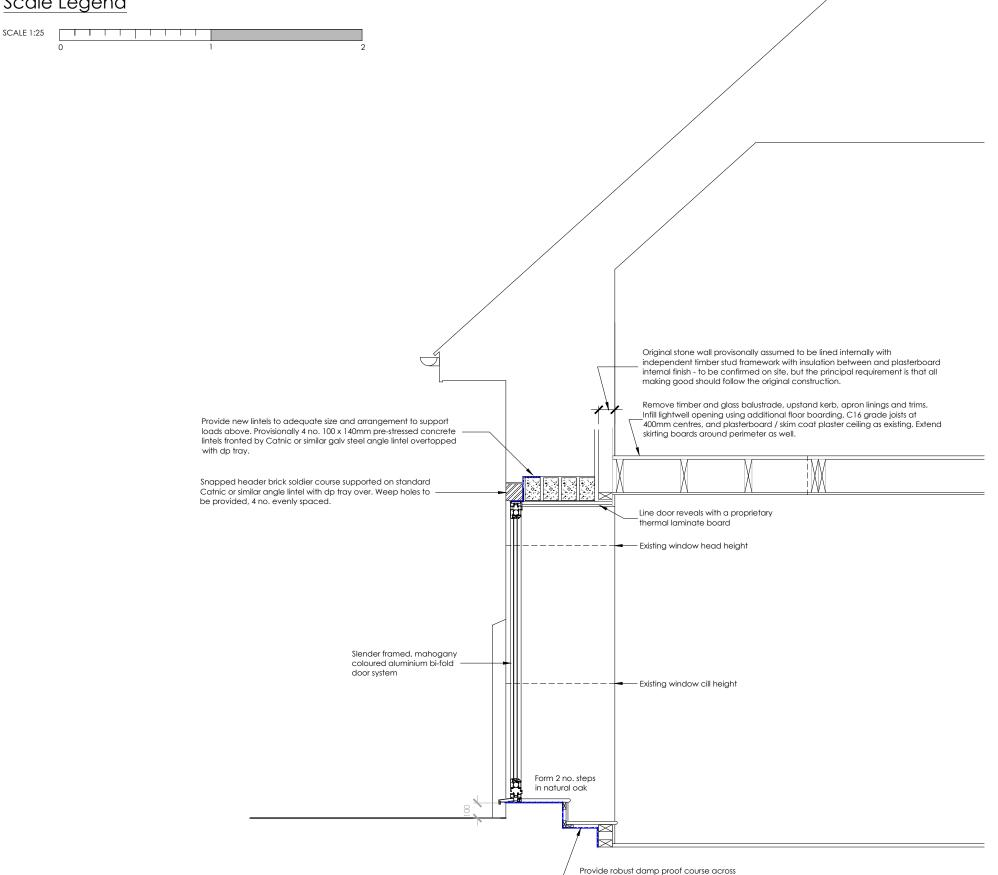
Provide robust damp proof course across new opening, fully sealed with existing dpc / waterproof membrane
