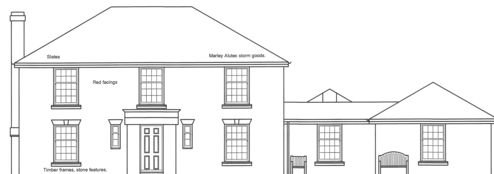
SOUTH WEST ELEVATION.
