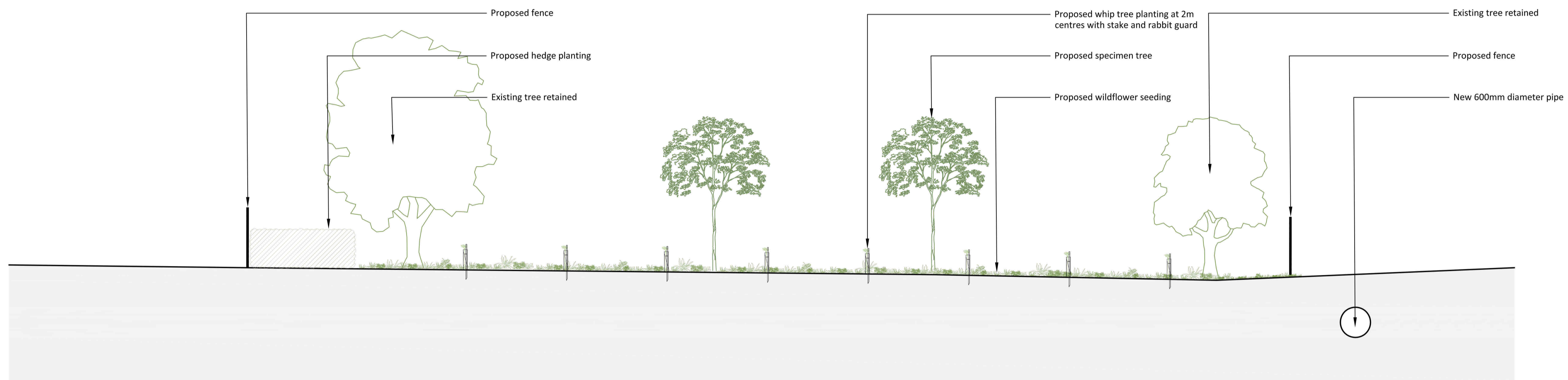
Section A-A Pipe installation & proposed mitigation planting
