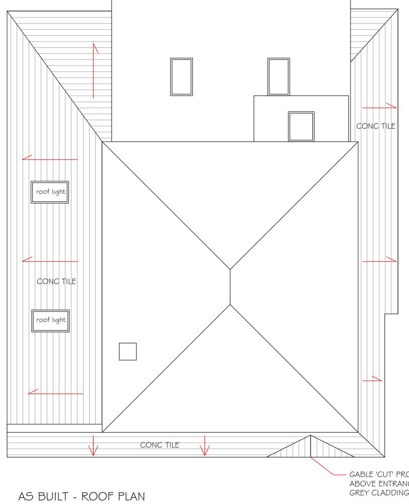
– GABLE 'CUT' PROFILE TO NEW ROOF ABOVE ENTRANCE DOOR GREY CLADDING TO GABLE INFILL
