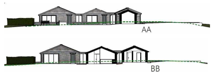
Figure 6: Changes in site levels
