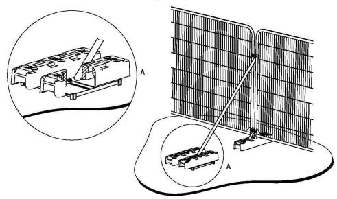
b) Stabilizer strut mounted on block tray
