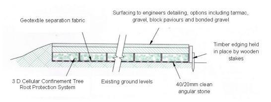
Illustration adapted from original drawings provided by Geosynthetics Ltd.
