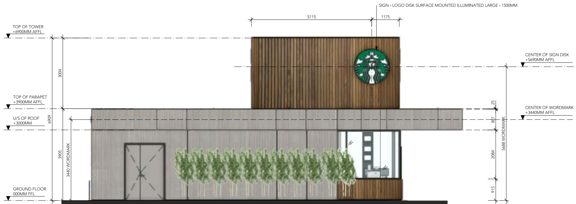
EXTERIOR ELEVATION - LEFT SIDE OF STORE Scale: 1:100
