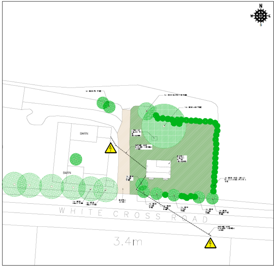
EXISTING SITE PLAN (1:200) CONCRETE PAVING (GRID PATTERN) KERB (DOTTED PATTERN) WHITE BRICK LAWN TREE GRAVEL TARMAK
