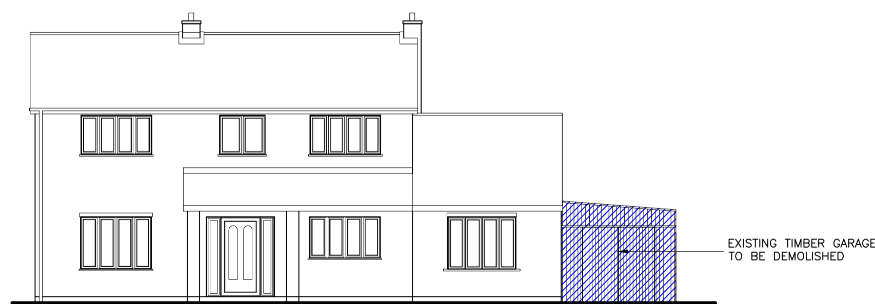
EXISTING FRONT ELEVATION (1:100)
