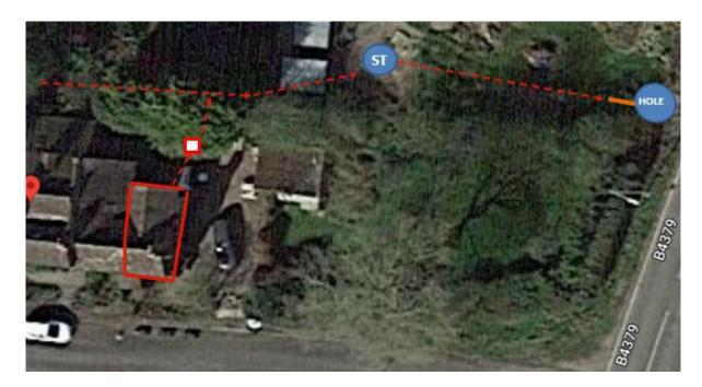
The foul waste only from both properties runs in to an old 3 chamber brick built system that is in a poor state of repair and not suitable or cost effective to be 'upgraded' to a more future-proofed and legislatively compliant system. (See images below – blue section is the approx location of the first chamber)
