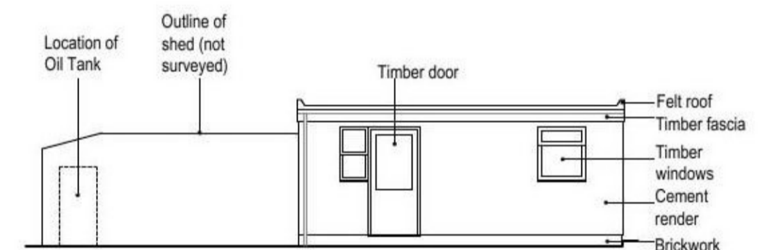
GARAGE WEST ELEVATION (AS EXISTING)
