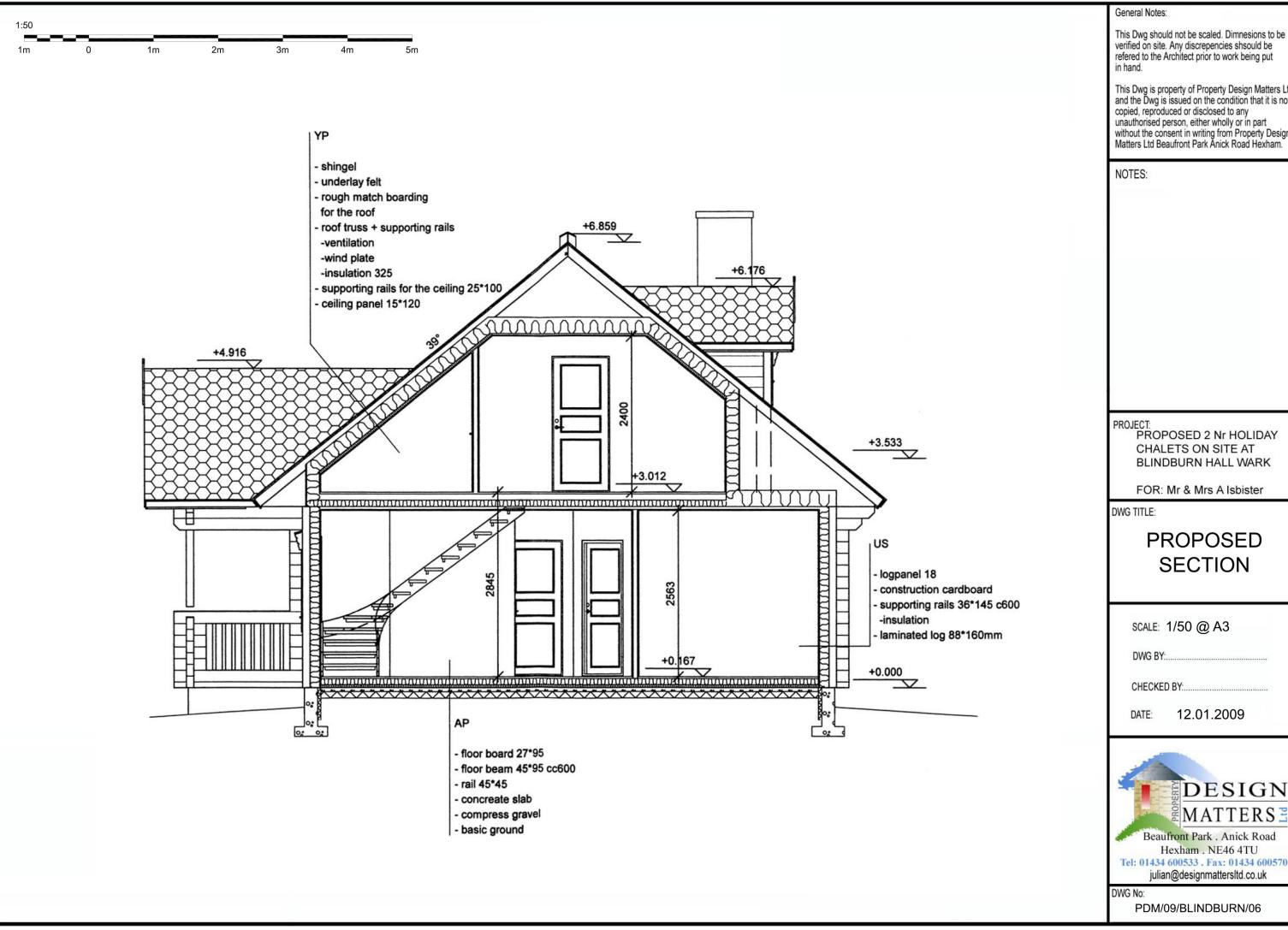
This Dwg should not be scaled. Dimnesions to be verified on site. Any discrepencies should be refered to the Architect prior to work being put
