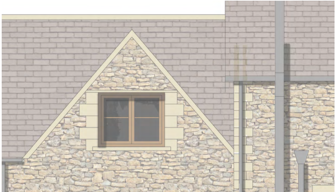
Example of typical Cotswold dormer with stone wall and timber casement window
